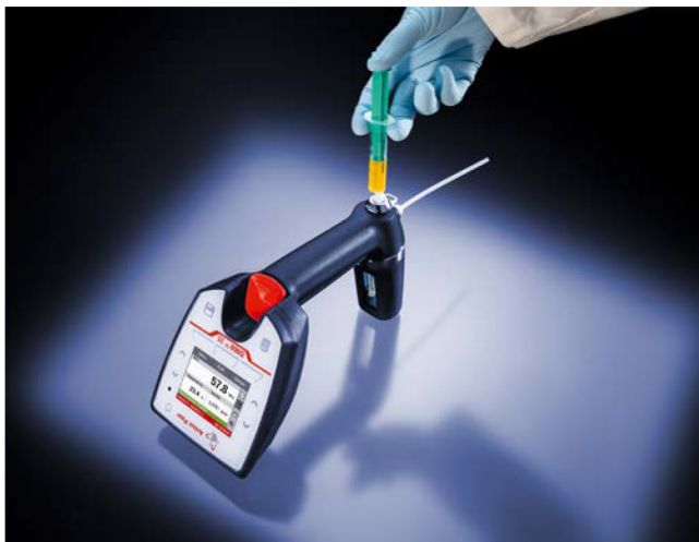
Figure 3: Filling DMA 35 Ex Petrol with a syringe
